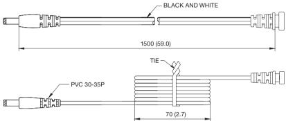
Wire type: VW-1 80°C 300V L=1500mm 2468 20AWG for 5 V output, 22AWG for 9V ouput, 24AWG for 12 V output, 2C Black and White. Black - Negative, White - Positive
