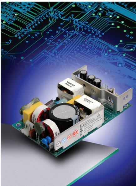
*The 3" x 5" CLC175 AC/DC power supply from XP Power is capable of delivering its 175 W full load output with only 10 CFM airflow*
