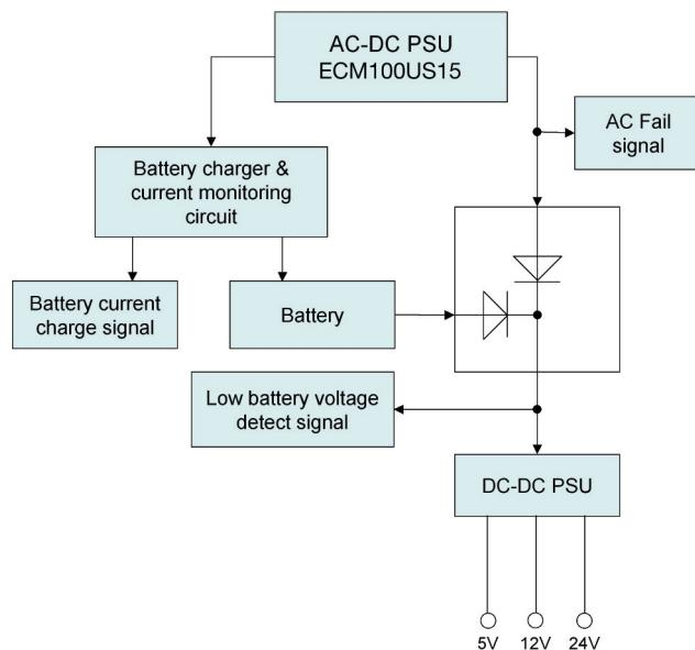
Earth leakage current was limited to 0.27mA in this application at 264VAC, 60Hz. The power supply meets EN60601-1, UL60601, and CSA-C22.2 No 60601.1 safety specifications and EN55011 Class A with respect to conducted emissions. It also complies with EN60601-1-2 (clause 36.22) and EN61000-3-2 with respect to EMC immunity.
