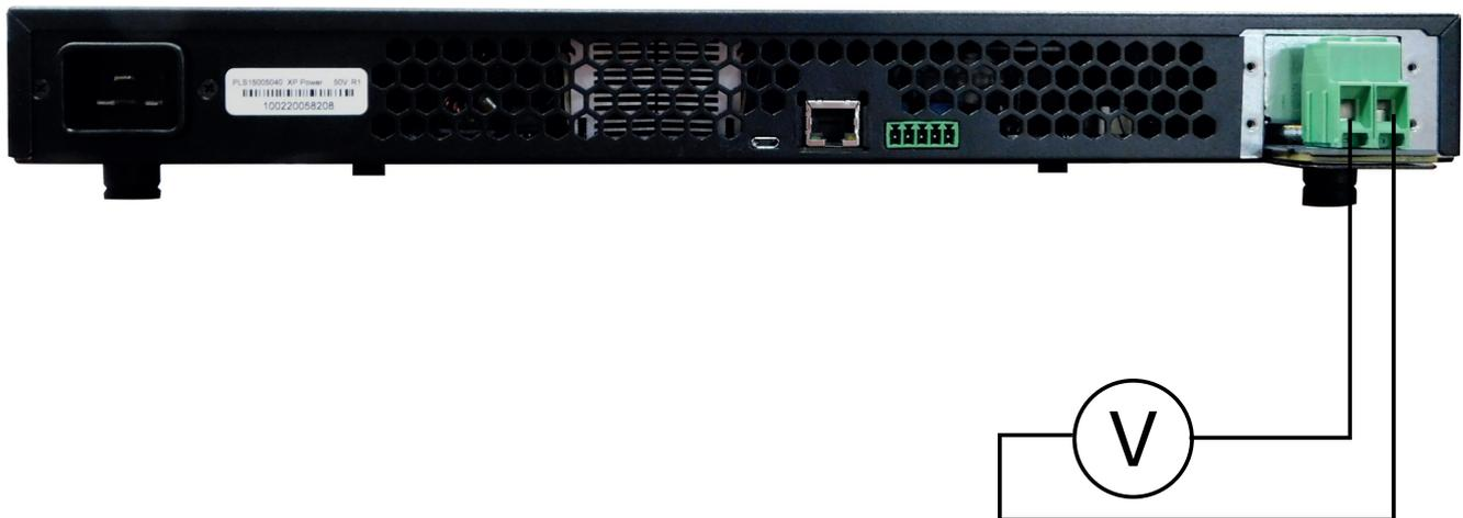
When the volt meter is connected, press the output on/off button. The following screen is an example of what will appear.
