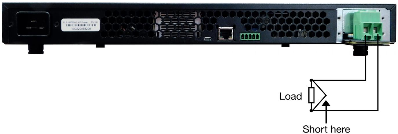
It is important that a good short with heavy wire is made as failure to do this will result in a poor remote sense calibration.
