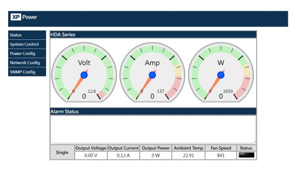
▶ 7.0 In the "Power Config" page, you will be able to change the settings of the power supply or devices. Make sure to press "Save Config" to save the settings.
