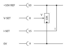
External potentiometer for current and maximum voltage.
