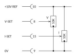
External potentiometer for voltage and maximum current.
