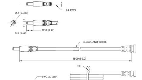
Wire type: VW-1 80°C 300V L=1500mm 2468 24AWG for 12V output, 2C Black and White. Black - Negative, White - Positive
