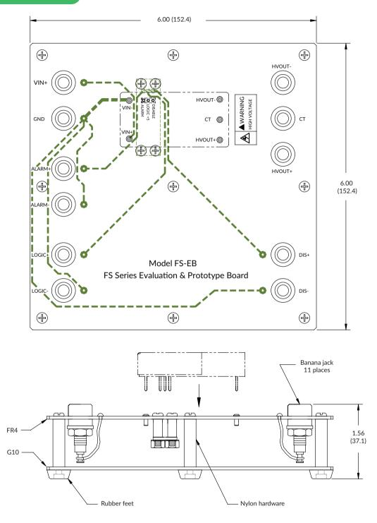
This FS-EB evaluation board provides a convenient package to use any FS Series high voltage power supply without having to it onto a PC board. The board provides for easy prototyping and evaluation. Please note when ordering, the FS Series unit is not included and must be ordered separately.
