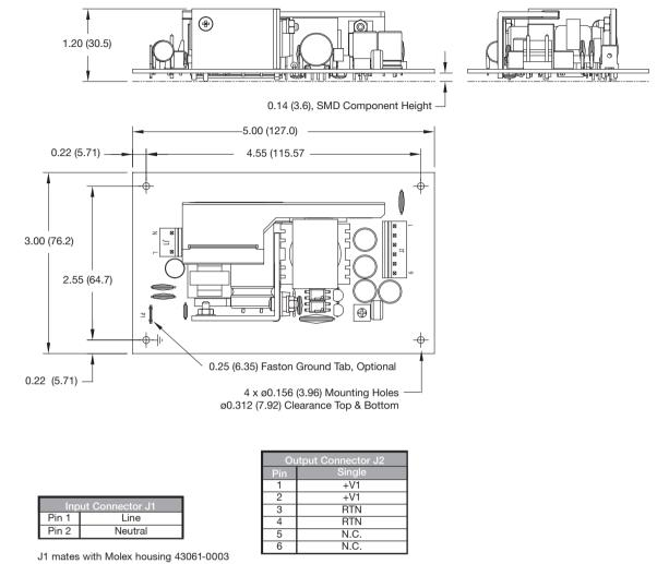
and Molex series 5194 crimp terminals. Ground (0.25 faston) tab standard.
