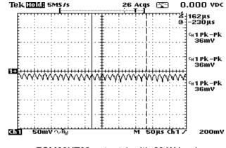
ECM60UT33 output 1 with 30 W load. Noise measured is 36 mV pk-pk
