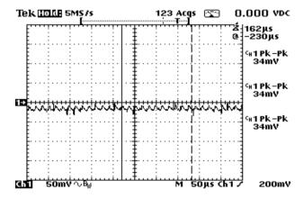
ECM60UT33 output 3 with 7 W load. Noise measured is 34 mV pk-pk
