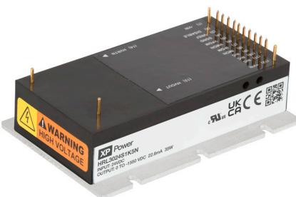
We offer a broad range of high voltage DC-DC products with output voltages from 100V to 25kVDC in both proportional and regulated outputs for high voltage applications. These DC-DC converters are highly controllable, high density, encapsulated, PCB mount, low noise power supplies generating a high voltage output that is fully controllable using standard low voltage circuitry.
