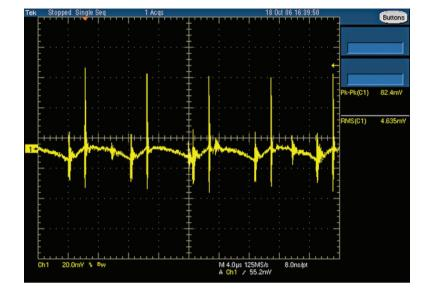
Figure 6 V1 MFA350PS12 (full load) 80 mV pk-pk ripple. 20 MHz BW
